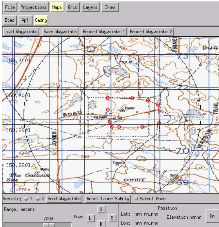
Figure 5: A high level path supplied via a user control station.
