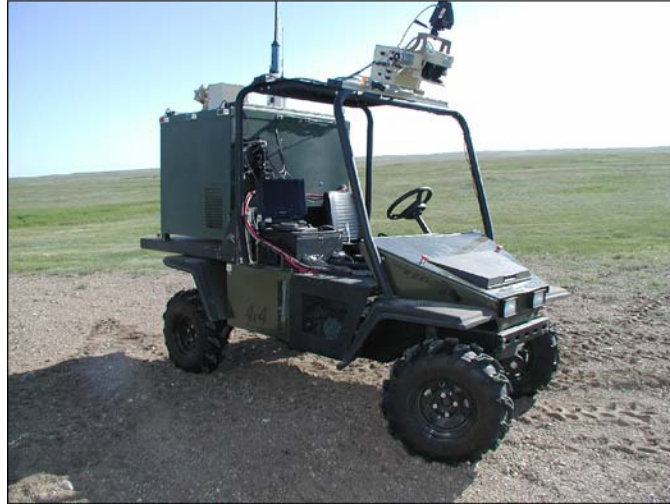
Figure 10: The Raptor UGV used to test the implementation of the Pure Pursuit algorithm.
