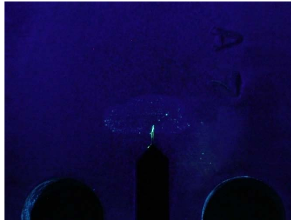
Residual Penetrant, 0X
