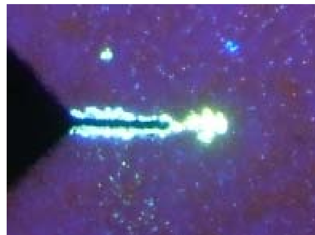
Notch and Crack at 60X
