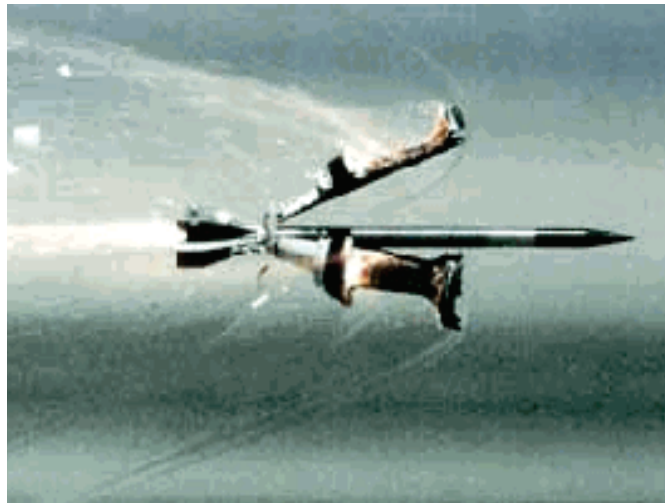
Figure 2-1. Sabot structure separating from DU penetrator.
