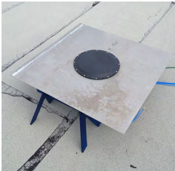
Figure 5. CRPA Antenna with an aluminum ground plane
