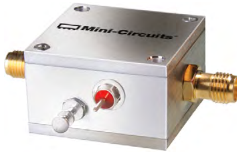
Figure 9. Mini Circuits ZFL-2500+ LNA (Figure provided by [8])
