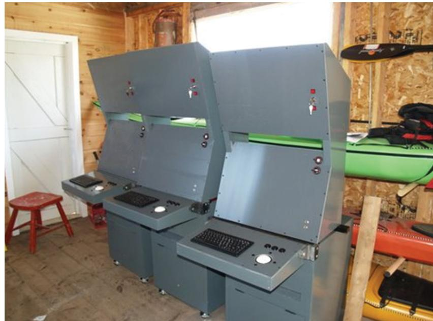
*Figure 1 Three Multi Function Consoles (MFC's) with keyboards and trackballs fitted.*
