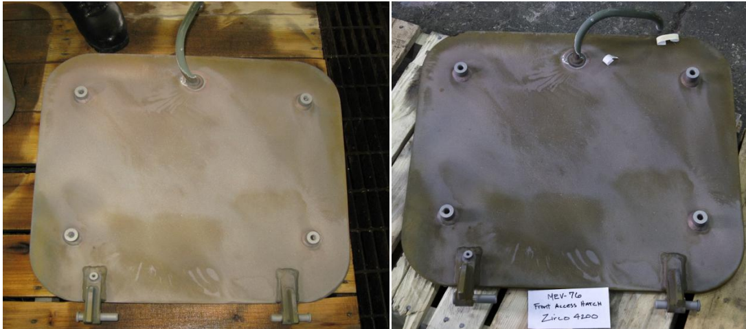
Figure 17. Front access hatch pretreated with PPG Zircobond 4200 immediately after pretreatment (left) and after approximately 19 h of ambient indoor exposure (right).
