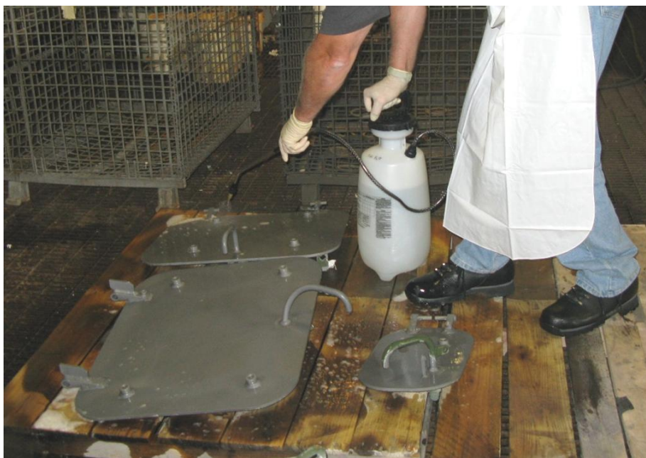
Figure 16. Actual application of the steel conversion coating on high hard Stryker hatches.
