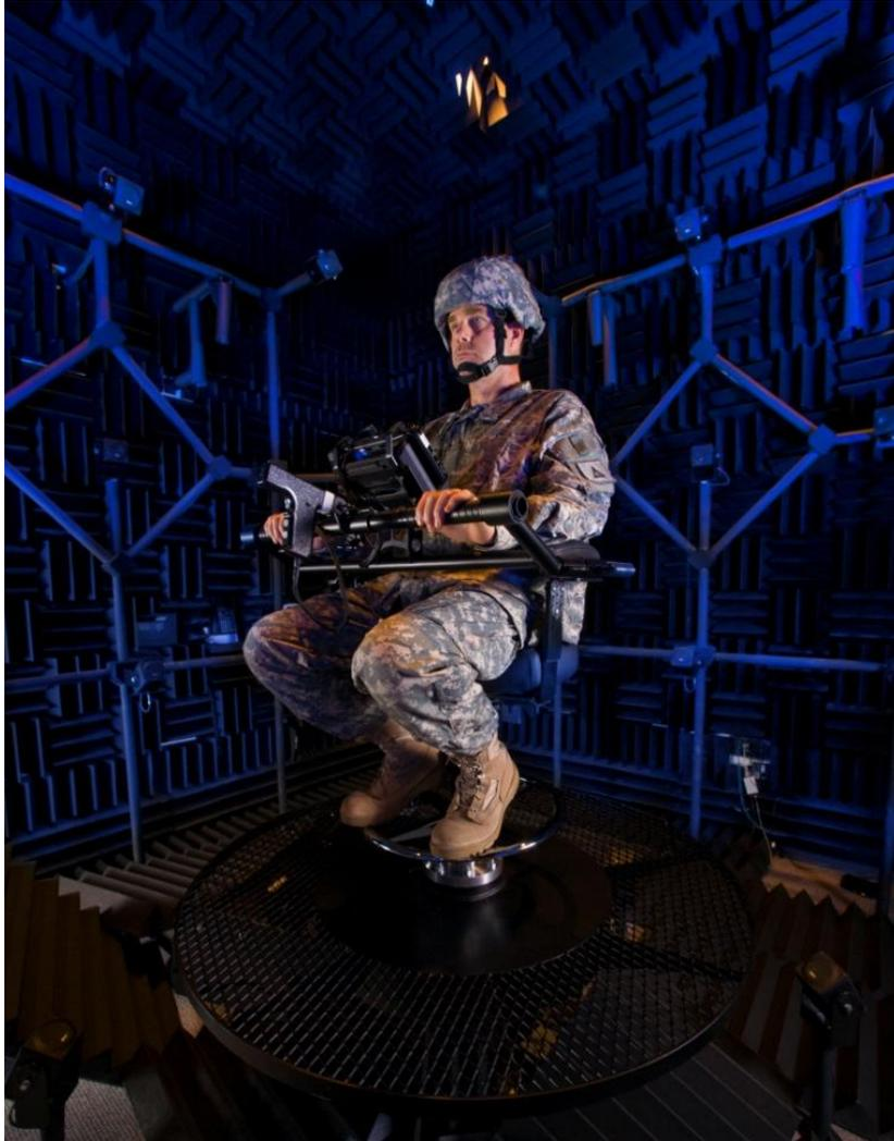
Figure 9. Testing setup used for the localization test. (No helmet used in this experiment.)
