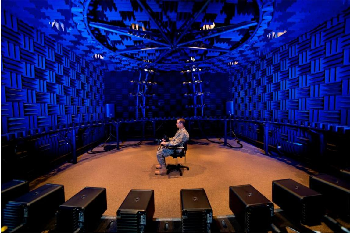
Figure 3. Dome Room of the Environment for Auditory Research at the U.S. Army Research Laboratory. (Person and chair shown were not present during recordings and were replaced by the G.R.A.S. 45CA shown in figure 2.)
