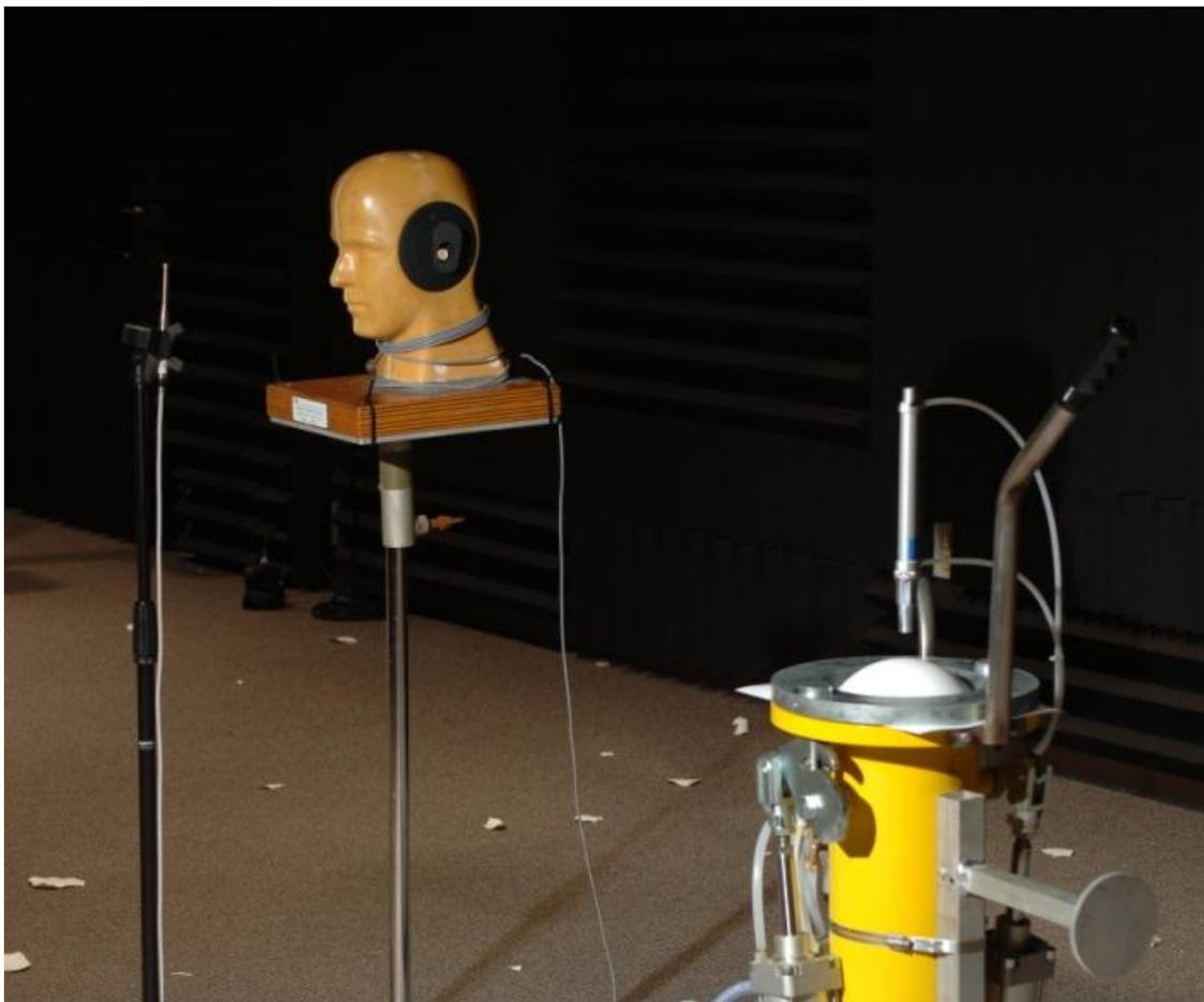
Figure 7. Left to right, G.R.A.S 40BH reference microphone, Institute Saint Louis (ISL) auditory test fixture, and shock tube used for impulse testing.
