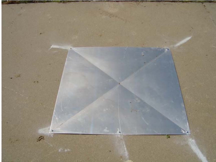
Figure 4: Aluminium witness plate.
