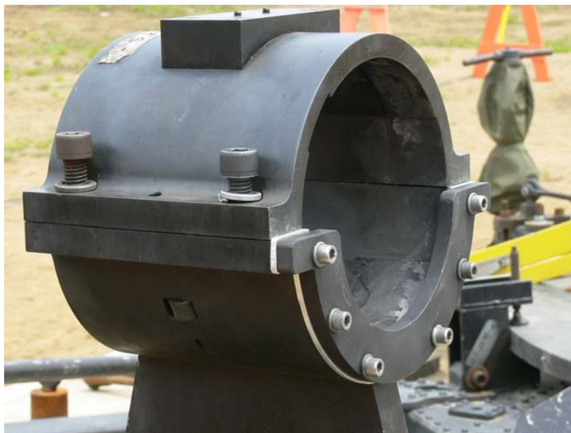
Figure 18: MK-58 motor collar.
