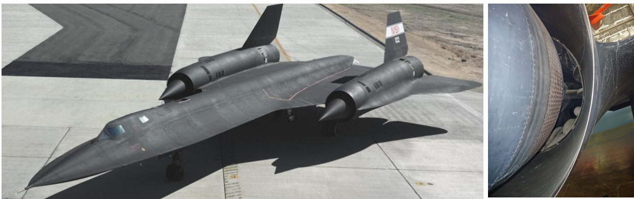
Figure 16: An SR-71 at Edwards courtesy of NASA and a close up of the spike and cowl internals of the YF-12 in the USAF museum courtesy of J. Kurzke.
