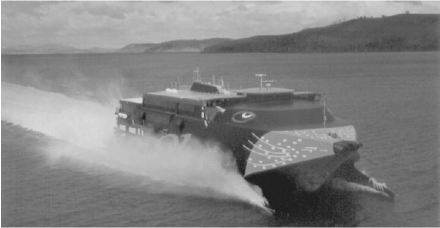
Figure 2.7 91-Meter Wave Piercing INCAT-046 Running at 43 Knots
