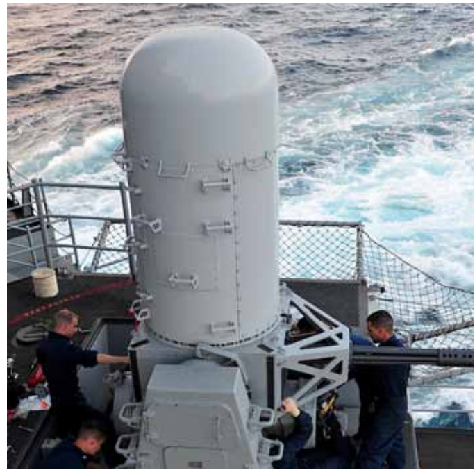
Sailors conduct routine maintenance on a close-in weapon system (CIWS) aboard an aircraft carrier. (U.S. Navy photo by Mass Communication Specialist 2nd Class Timothy M. Black/Released)
