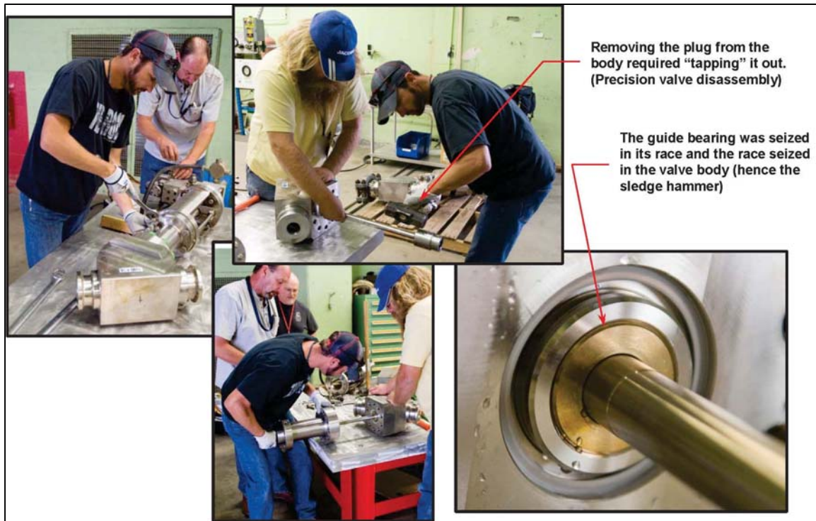
Figure 3. Removing the plug from the valve body was very difficult. We would not usually use a sledge hammer to get the plug/stem assembly out of the valve.
