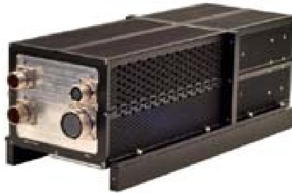
Figure 6. The avionics box contains the combined GPS/INS (front two-thirds) and the TSAS electronics (rear one-third) for a fully self-contained system to permit flight testing in legacy aircraft with minimal avionics or lacking 1553 / ARINC connectivity. The interfaces on the front include connections for 1553 and/or ARINC bus, power, pilot control unit and outputs to TSAS seats, torso garment, and shoulder harness.
