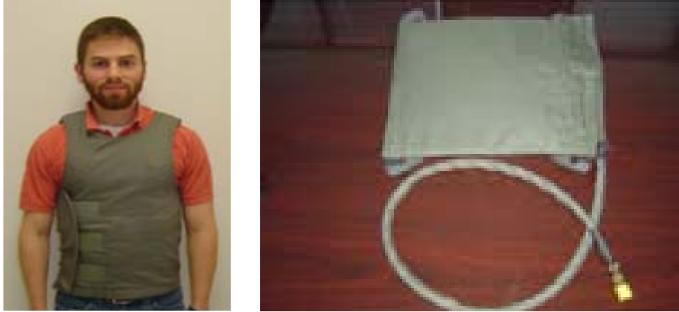
Figure 5. The full torso garment (left) is fitted with a distributed factor system, and the seat cushion (right) is fitted with eight additional factors before incorporation into the H-60 seat cushion.
