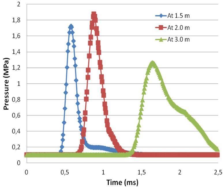
Figure C-2: Incident pressure for a rectangular mesh with element size of 75 mm at 1.5 m, 2.0 m and 3.0 m.
