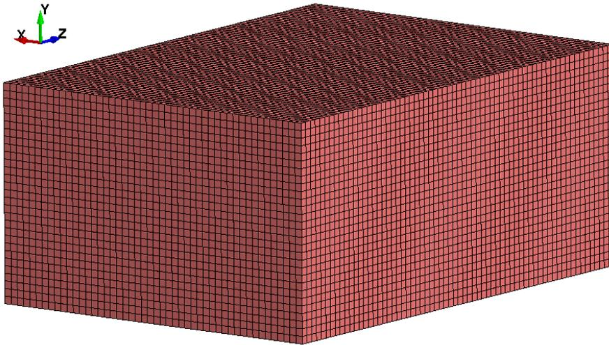
Figure 2: ALE rectangular mesh<sup>5</sup> with element size of 200 mm
