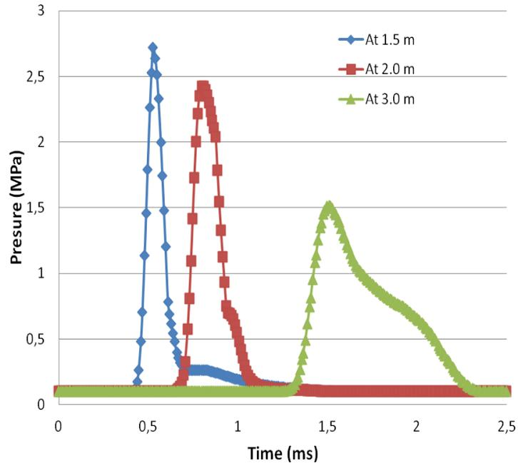
Figure C-3: Incident pressure for a rectangular mesh with element size of 50 mm at 1.5 m, 2.0 m and 3.0 m.
