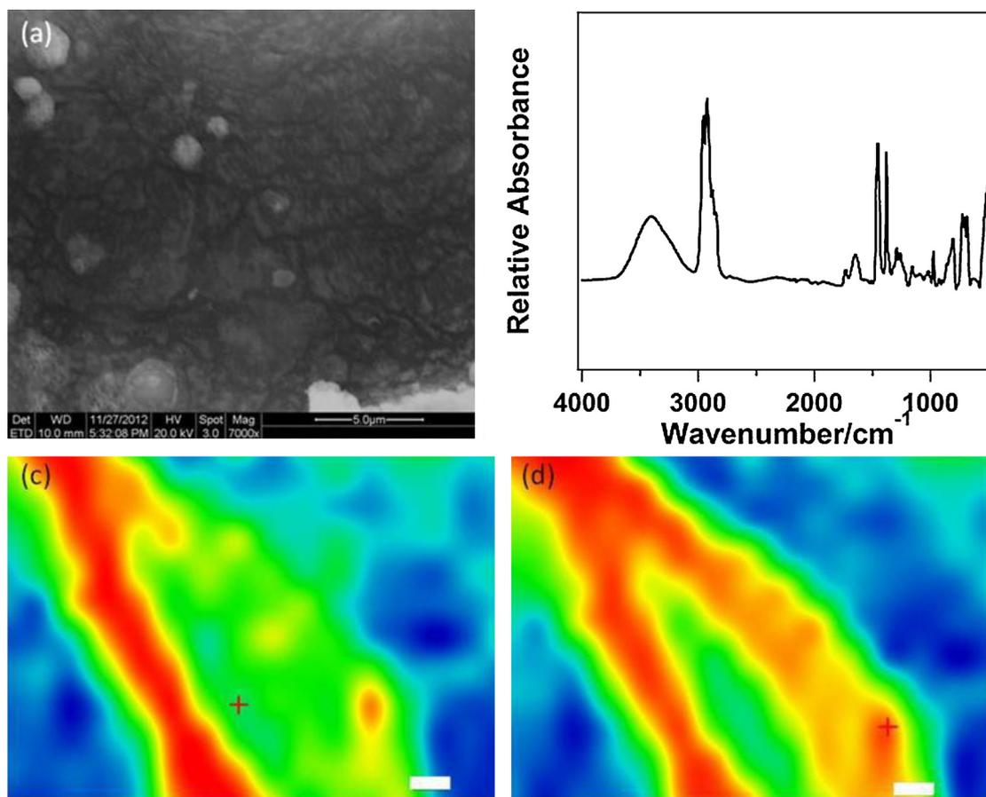
**Fig. 5.** (a) ESEM image of cast membrane surface, (b) FT-IR spectrum of the quaternized membrane, (c) contour plot of  $3600\text{ cm}^{-1}$  wavenumber intensity with  $100\text{ }\mu\text{m}$  scale bar, (d) contour plot of  $2900\text{ cm}^{-1}$  wavenumber intensity with  $100\text{ }\mu\text{m}$  scale bar.
