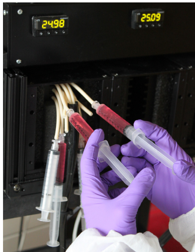
Fig. 2. Multiple fluidic biochips inserted into the multichannel reader test unit for 1 h exposure testing. The picture depicts a manual exposure injection with attached syringes of control and test samples in L-15ex media.
