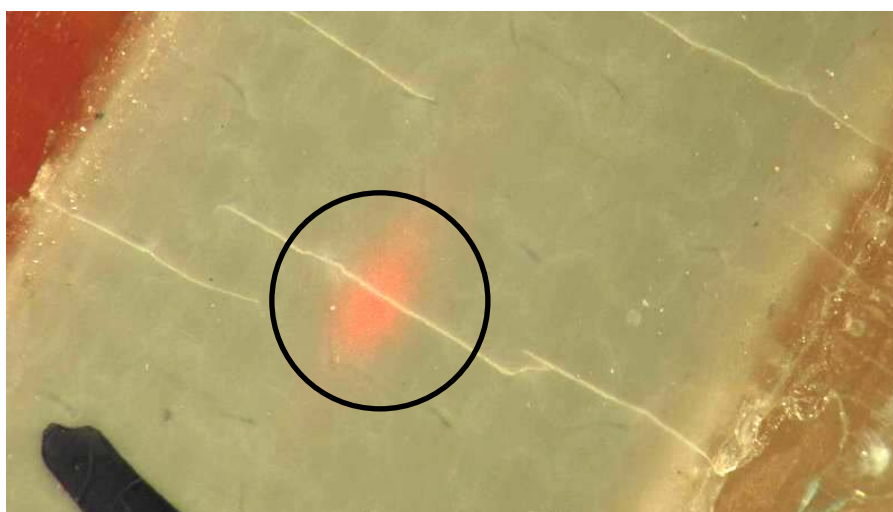
Figure 7.5: Fractures in Redux packaging. The red light seen in the highlighted region in the centre of the patch is the visible source escaping at the point of fracture in the optical fibre.
