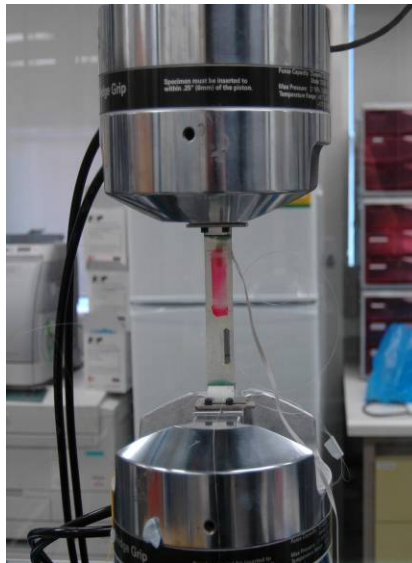
Figure 5.12: Test coupon with surface mounted FBGs in a 50 kN MTS system.
