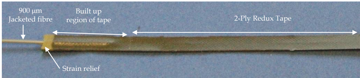
Figure 2.6: Close-up of the cured Redux tape showing built-up egress point of jacketed optical fibre from Redux tape.
