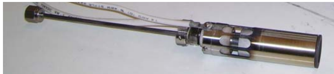
Figure 3. Busek’s 1.3-cm hollow cathode.
