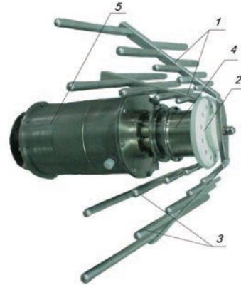
General view of beamless coaxial generator MG1 with connected capacitor storage (Length less than 0.5 m)
