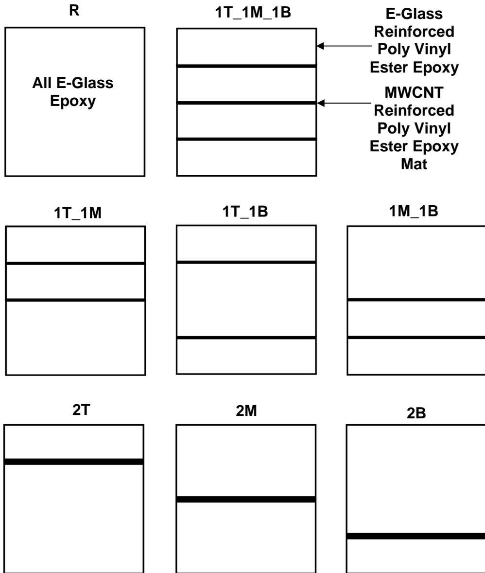
**Figure 2 Various hybrid-armor design configurations analyzed in the present work.**
