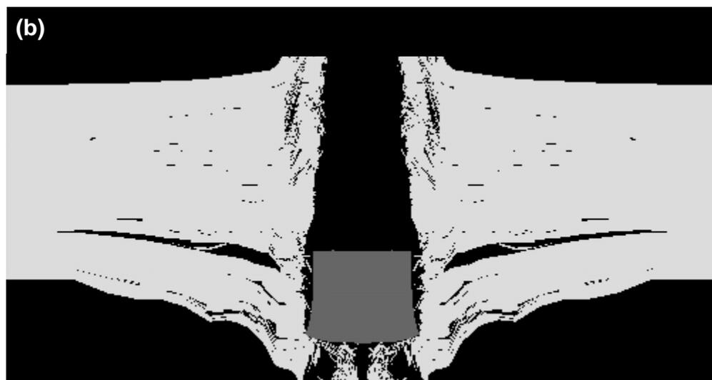
**Figure 4 Experimental (a) and computational (b) material distribution/damage results pertaining to the impact of a 0.50 caliber FSP with a 25.4 mm-thick all E-glass continuous-fiber reinforced poly-vinyl-ester-epoxy matrix composite armor. Initial projectile velocity, 605 m/s.**
