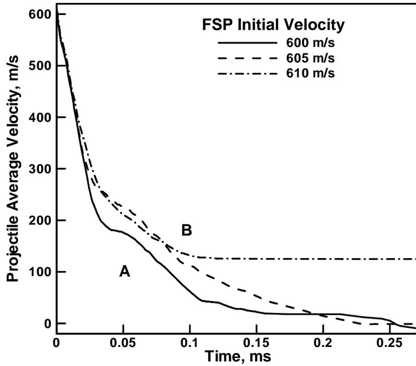
**Figure 3** Temporal evolution of a 0.50 caliber FSP velocity during the impact with a 25.4 mm-thick all E-glass continuous fiber-reinforced poly-vinyl-ester-epoxy matrix composite armor.
