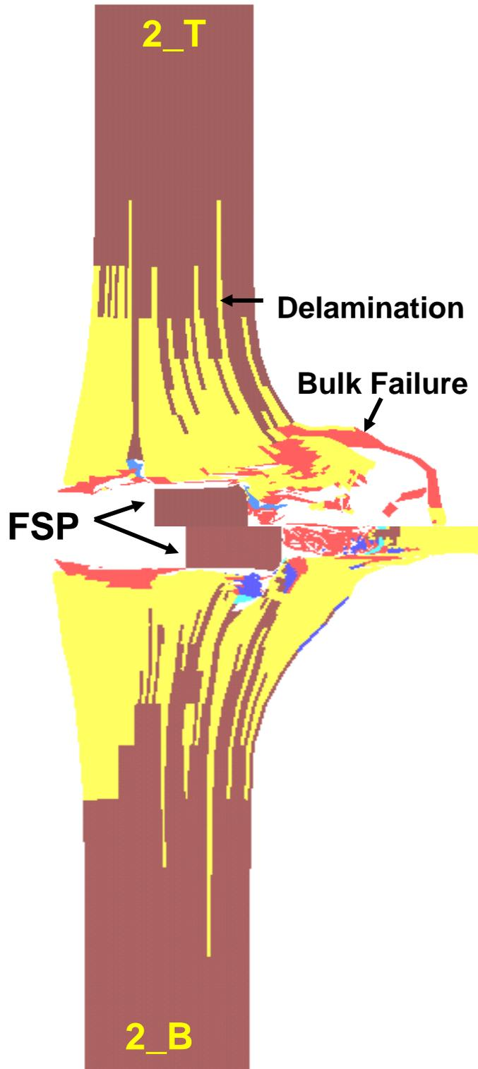
**Figure 6. A comparison of the material deformation/failure status plots for the 2\_T and 2\_B hybrid armors at the same projectile post-impact time of 0.04ms. It should be noted that the axis in this figure is rotated by 90 degrees relative to those used in Figures 1, 2 and 4.**
