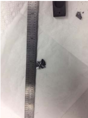
Figure 4: C12A7 electride insert pieces for a second generation prototype hollow cathode.
