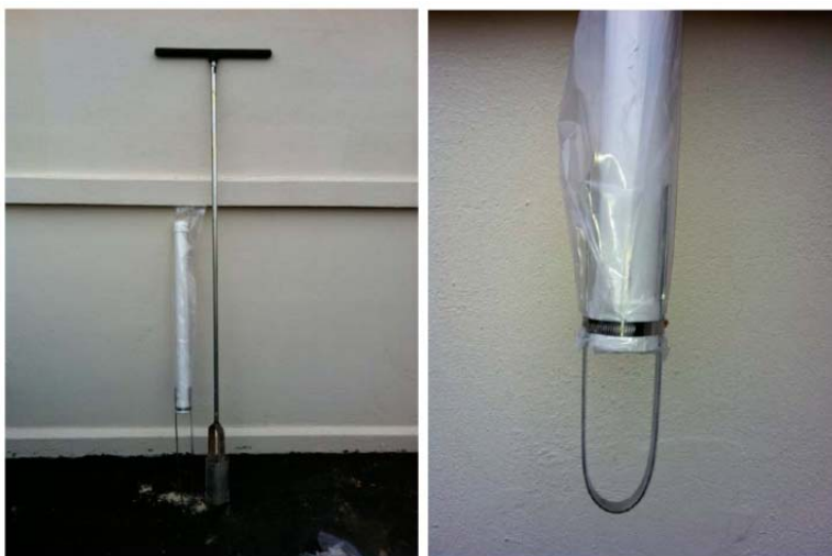
Figure 24. Passive soil gas probe showing aluminum stilts used to suspend the pipe above the bottom of the augured hole and the plastic sleeve that was filled with tamped sand to seal the borehole annulus, both of which are secured with a stainless steel ring clamp.
