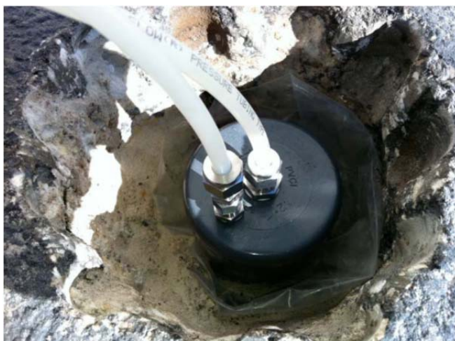
Figure 25. Cap of passive soil gas probe with fittings for purging line (extends to just below cap) and Summa™ canister sampling line (extends through 1/8-inch stainless steel tubing to bottom of PVC pipe).
