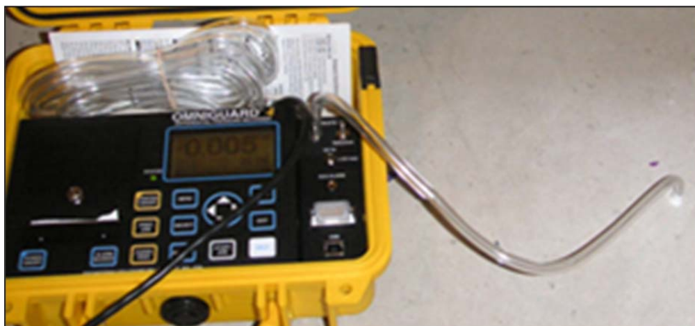
Figure 29. Set-up for cross-foundation measurement with a pressure transducer. Note that reference port is located to the right-hand side of the sub-slab connection on the Omniguard transducer.
