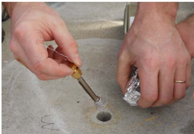
Figure 23. Deployment of a fully passive ATD tube sample showing wire basket used to prevent contact with soil at the bottom of the cored hole, steel wire tether for retrieval, and rubber stopper wrapped in aluminum foil used as a temporary cap.
