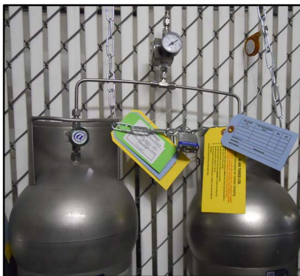
Figure 6. Setup of a pair of Summa™ canisters connected to a single intake valve used for demonstration. For size comparison, a 3M OVM 3500 passive sampler is on the top-right corner.
