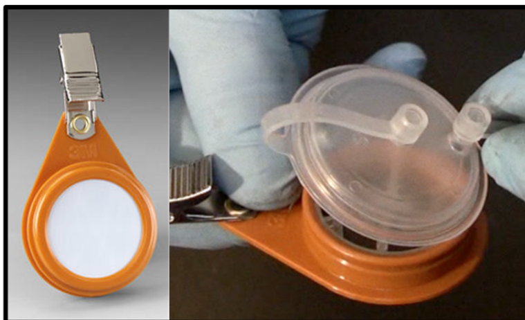
Figure 3. 3M OVM 3500 passive sampler showing solid plastic cap used to replace a porous plastic sheet after sampling is complete.
