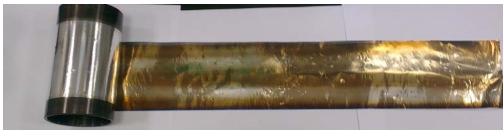
Figure 10. the photo of PBT-Al after roll-calcination process.
