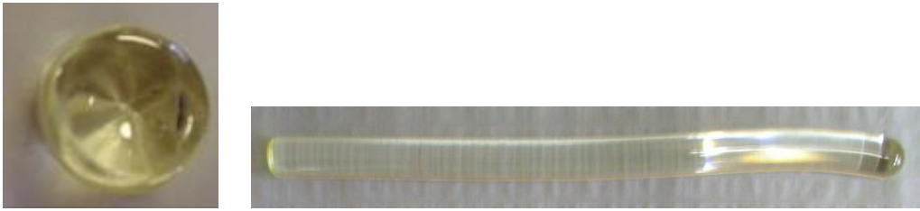
Figure A.16: (Left) 3cm diameter lead-germanate glass billet made from 150g batch and (Right) extruded rod of 1cm diameter and 16cm length made using this billet.
