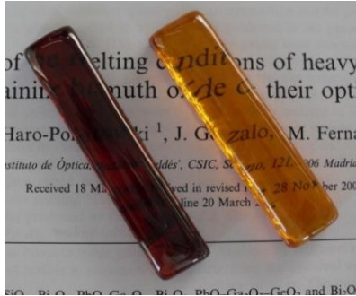
Figure A.7: Photographs of 70 \text{GeO}_2 - 25 \text{Bi}_2\text{O}_3 - 5 \text{WO}_3 glasses without \text{CeO}_2 (left) and with 0.1 \text{CeO}_2 substituted for \text{GeO}_2 (right).
