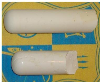
Fig. 55 — Photographs of 50% DEB monolith as-synthesized (top) and following Soxhlet extraction with 1 M HCl in ethanol for 5 days (bottom)
