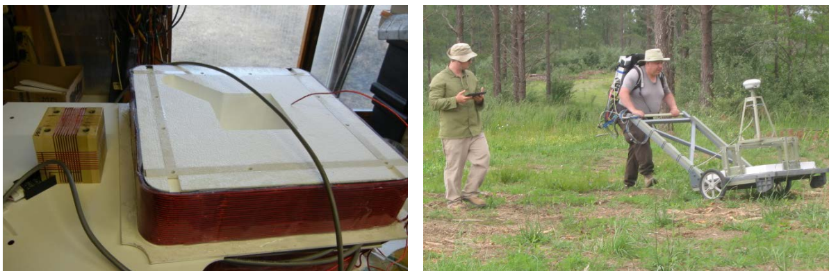
Figure 2-1 – Left: Individual TEMTADS/3D EMI sensor with 3-axis receiver under construction, Right: Man-portable TEM array with GPS antenna.
