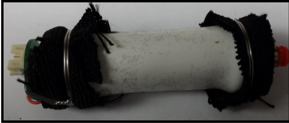
Figure 44 - Gripper after 47,097 successful cycles.
