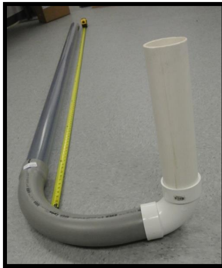
Figure 3- 3 in. Mock piping
