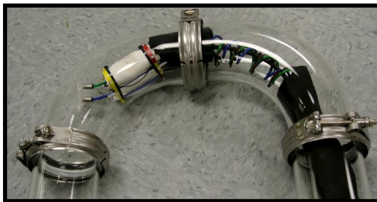
Figure 14 - Navigation through inline elbows test
