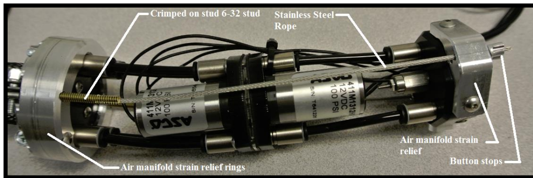
Figure 33 - Steering head assembly
