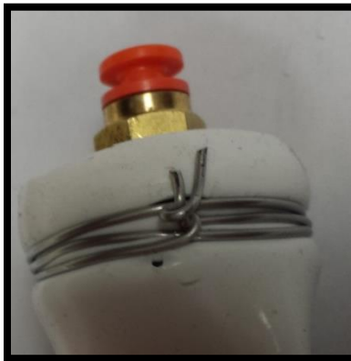
Figure 43 - Gripper silicone failure
