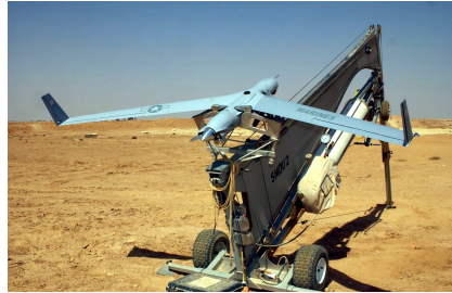
(a) ScanEagle 3m wingspan 13kg empty
