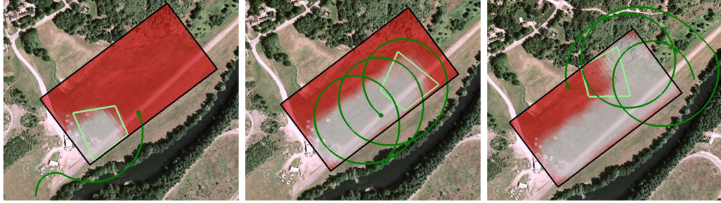
Figure 5.2: Several coverage snapshots from a search of a typical open rectangular area. The level of coverage is indicated by red shading, with completely uncovered areas displayed in the darkest shade of red, and sufficiently (exceeding an adjustable threshold on probability of detection) covered areas as white. The path of the UAV is drawn in dark green, its current location marked by a green dot, and the current sensor footprint as a light-green trapezoid.
