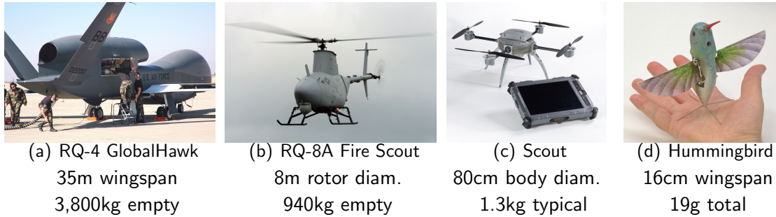
Figure 1.2: Several unmanned aircraft demonstrating a spectrum of portability roughly parameterized by the magnitude of vehicle size, weight, cost, feature set, flight altitude, mission duration, and launch facilities. These include (a) the Northrop Grumman RQ-4 Global Hawk, (b) the Northrop Grumman RQ-8 Fire Scout, (c) the Aeryon Scout, and (d) the AeroVironment Nano Hummingbird.
