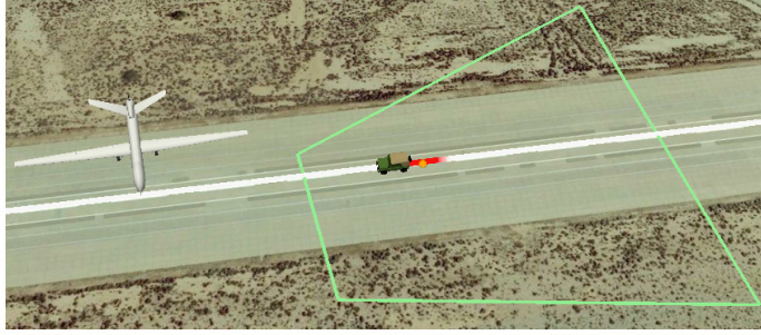
Figure 4.17: Visualization example from simulation showing a UAV pursuing a Jeep. The green trapezoid is the ground region visible to the camera. The orange dot indicates the geolocation filter’s best estimate of the target’s position at the center of the red smear denoting the surrounding uncertainty distribution.
