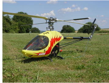
(b) Joker 2 1.8m rotor diam. 8kg loaded
