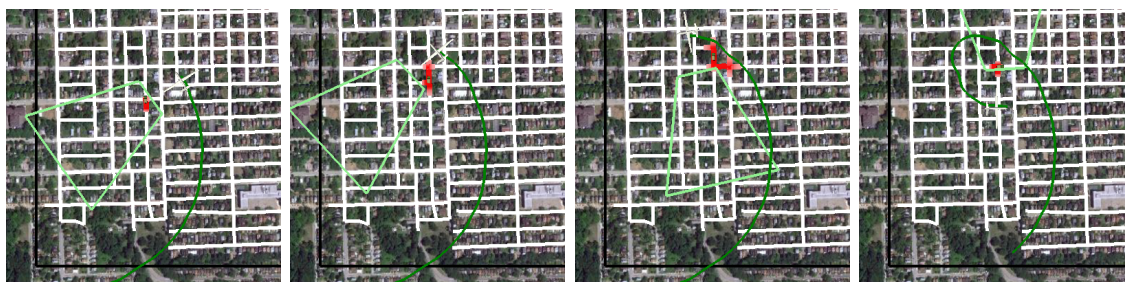
Figure 4.19: An example of pursuit in a road network using cellular decomposition. The UAV anticipates loss of view (area within the green trapezoid) and begins to turn sharply. While out of view, it predicts diffusion in possible target location (red probability mass) and greedily steers to maximize the probability of re-detection.
