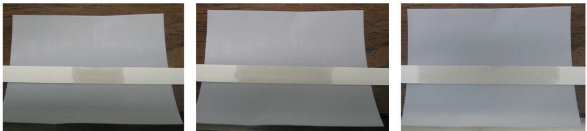
Figure 6: Oil sensing results by using a 290-mm long paper strip (different spread: 17, 34, 50 mm).
