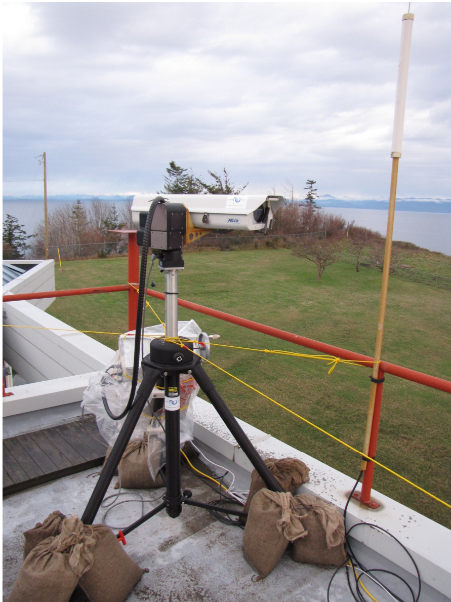
Figure 1: ASIA deployment during the 2010 Vancouver Olympics. The AIS antenna can be seen on the wooden pole to the right. The ASIA camera is contained within the Pelco enclosure (i.e., white case) on top of the tripod.
