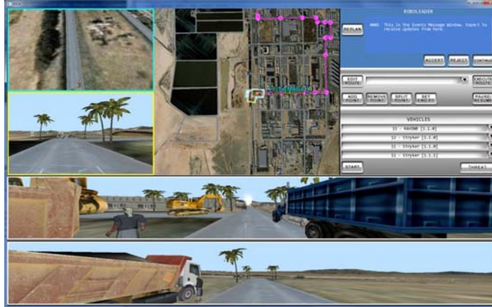
Figure 1. Operator control unit: user interface for convoy management and 360° tasking environment.
