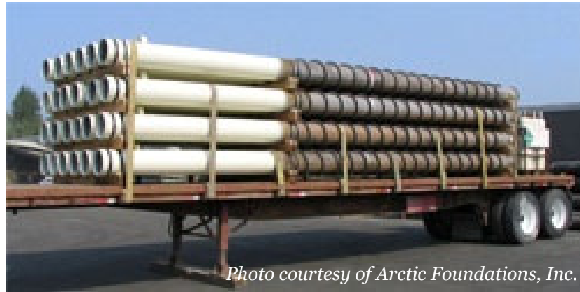
Figure 6. Thermo helix piles loaded for shipment.
