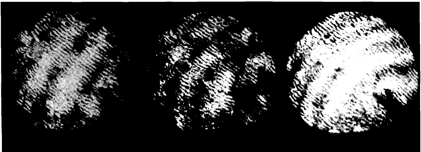
Figure 2. Interference fringes from which the coefficient of thermal expansion of Zerodur was determined.
