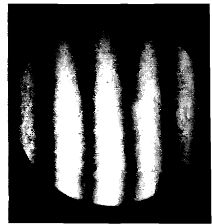
3 HOURS AFTER 150°C OVEN FRINGES VERTICAL
