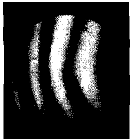
24 HOURS AFTER 300°C OVEN FRINGES VERTICAL
