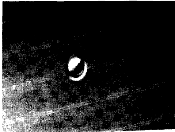
Figure 10. Higher magnification Nomarski micrograph of the small damage site shown in Fig. 9. This melt crater has a major axis of about 30 \mu\text{m} and was formed just at threshold.
