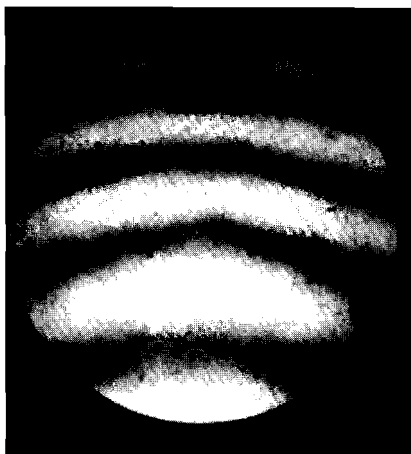
24 HOURS AFTER 300°C OVEN FRINGES HORIZONTAL
