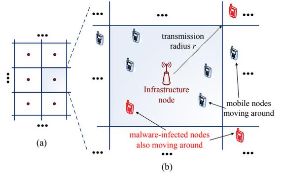
Fig. 1. Network architecture: infrastructure nodes and mobile nodes.
