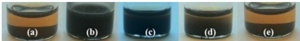
Figure 4.9.1 [1-Bu-3-Me-Im][4,5-DiCN-Im] with 0.093 % Ti: (a) before sonication, (b) immediately following sonication, (c) 24 h ( T_s ), (d) 30 h, (e) 36 h ( T_f ).
