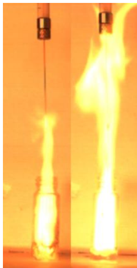
Figure 4.8.2 Enhancement of ignition observed from [1-Me-4-NH 2 -Tri][DCA] (left) to [1-Me-4-NH 2 -Tri][DCA] with 0.33% B (right)
