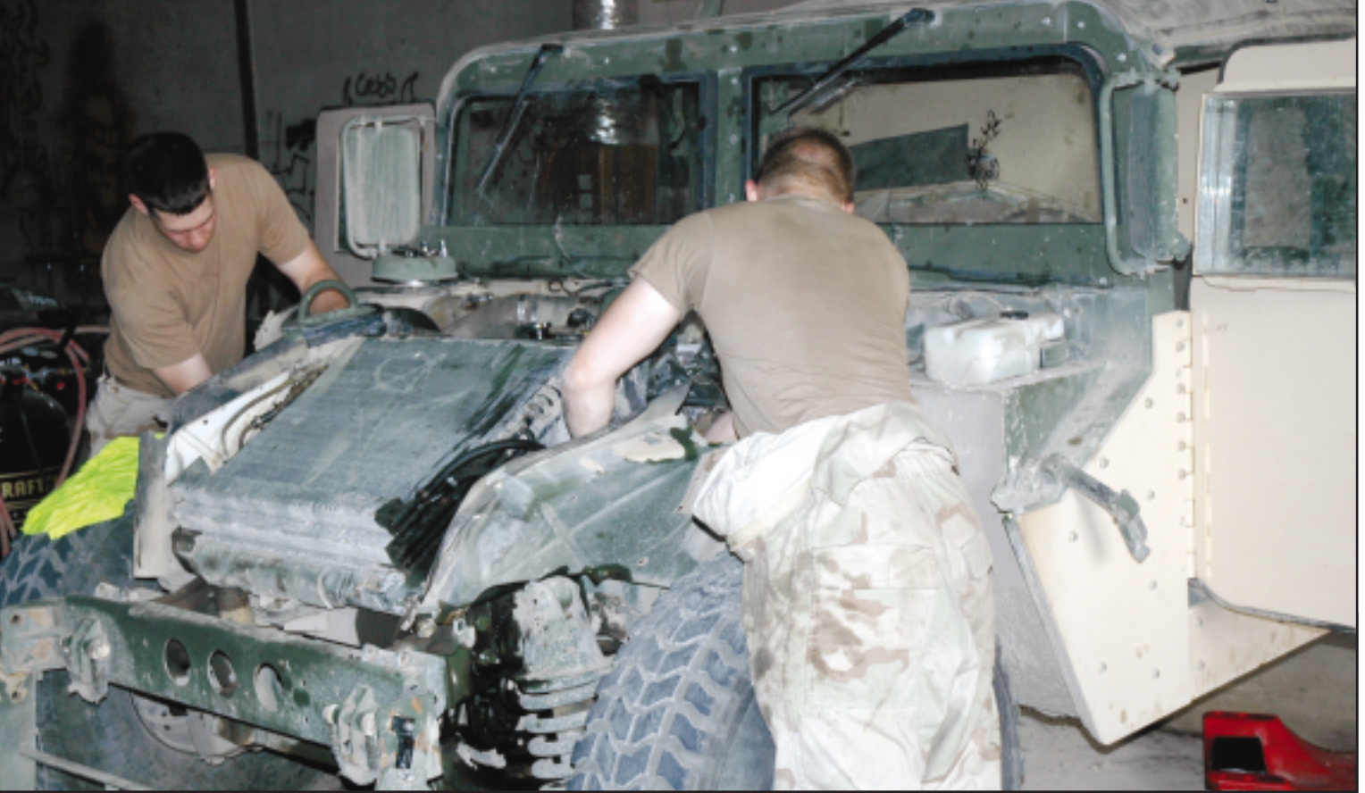
Two Soldiers from the 536th Maintenance Company, 17th Corps Support Battalion (CSB), 917th Corps Support Group, 1st Corps Support Command, repair a high-mobility, multipurpose, wheeled vehicle that was recovered after it was damaged by an improvised explosive device during a combat logistics patrol in Iraq. The 17th CSB, an Active Army unit from Schofield Barracks, Hawaii, is responsible for recovery of vehicles for corps units, multinational forces, and contractors in the Multinational Brigade Northwest area of operations. Recovery teams determine the severity of a vehicle's damage and then haul the vehicle to a place where further assessments can be made. If they cannot make repairs at that site, they move the vehicle to a maintenance site for repair. If the vehicle cannot be repaired, functioning parts are removed for use on other vehicles.
