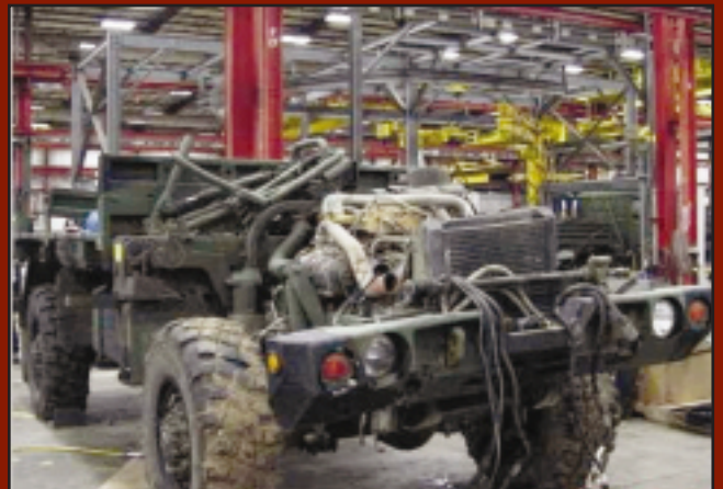
The first step in the repair process is to remove the cab and engine.
