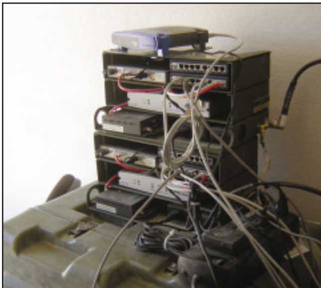
A CAISI is set up in a field environment (above). One main CAISI system in a unit is connected to the VSAT (below), and other elements that have CAISI systems can interface with the main CAISI to establish Internet connections.
