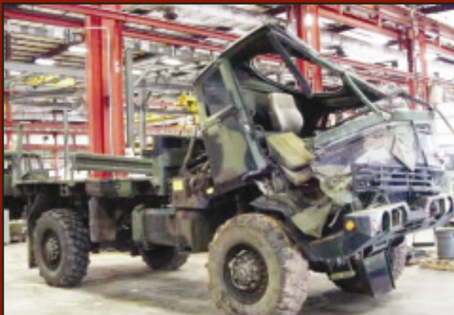
This M1081 standard cargo low-velocity-airdroppable truck needs considerable repair when it arrives at the reset facility.
