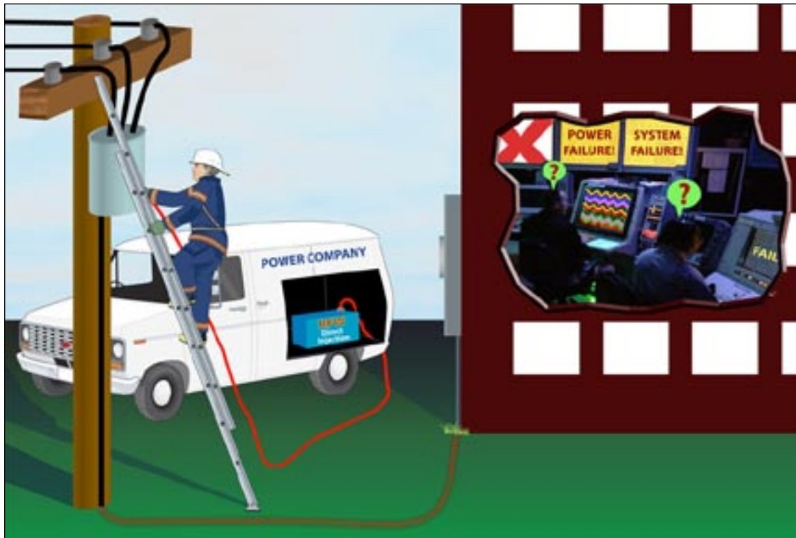
Figure 6 - Illustration of Conducted Threat from an RFW
