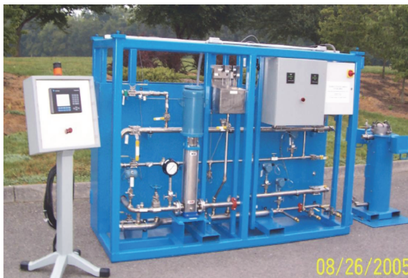
Figure 7-2. Pilot-scale prototype of RO system to remove RDX from munitions production wastewater.
