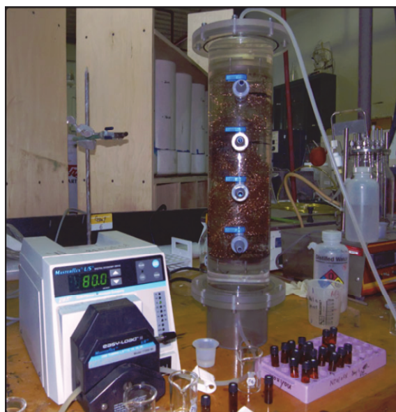
Figure 5-4. Upflow-through suspended iron particles reactor in operation.
