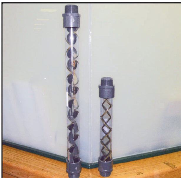
Figure 5-2. Six (11" long) and twelve (18" long) mixing elements plastic static mixers.
