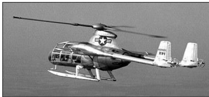
Figure 2, McDonnell Aircraft Corporation, XV-1, Unloaded Rotor Principal
