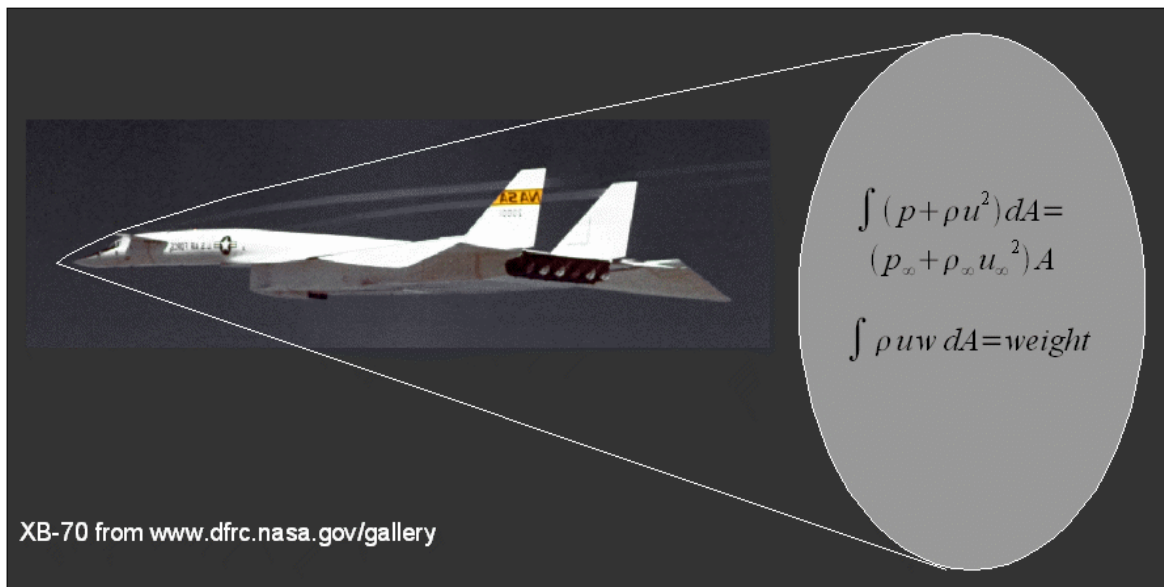
Figure 2 A control volume defined by the intersection of the bow shock and a vertical plane normal to the horizontal flight velocity vector.
