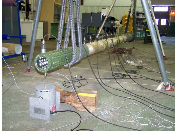
Figure 4: ATD-6 Modal Testing Setup
