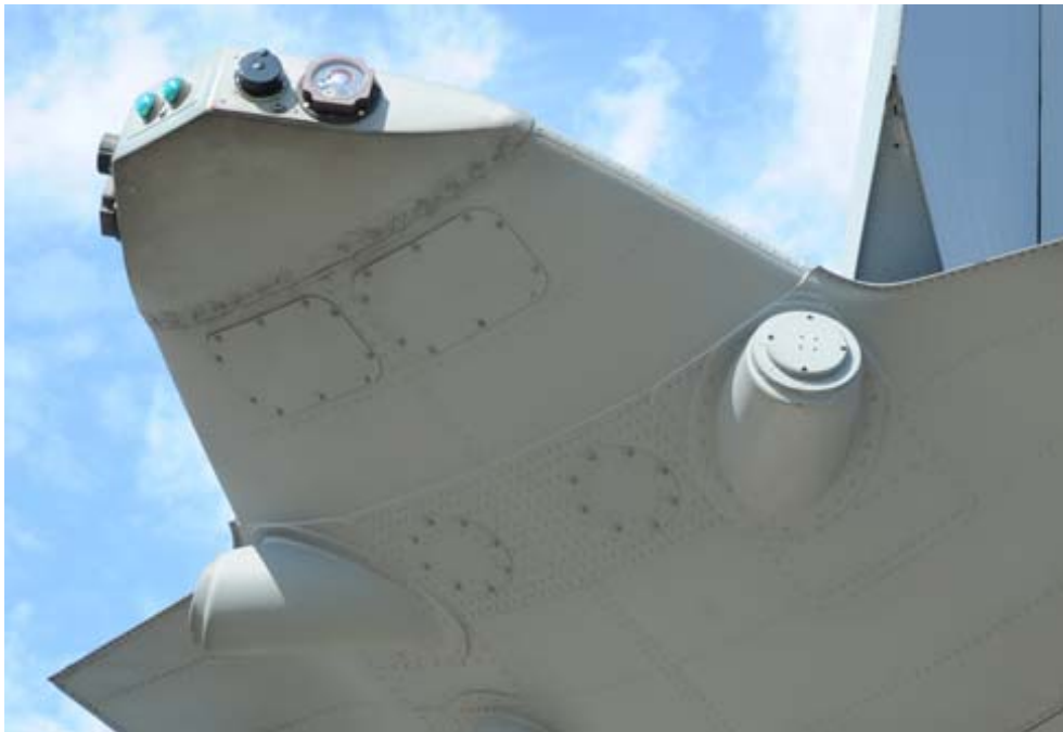
Figure 2-16: Top: AN/AAR-54 Electronic Unit and Sensors – (Courtesy of Northrop Grumman Corp.); Bottom: Aft Missile Warning Sensor Installation on a C-130 – (USAF Photo).
