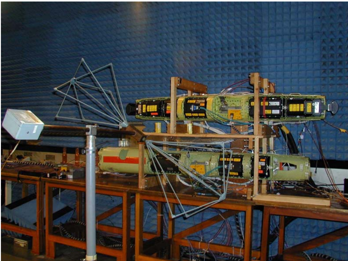
Figure 6-17: Typical EMC Testing of EW Equipment – (© BAE Systems 2003, All Rights Reserved).
