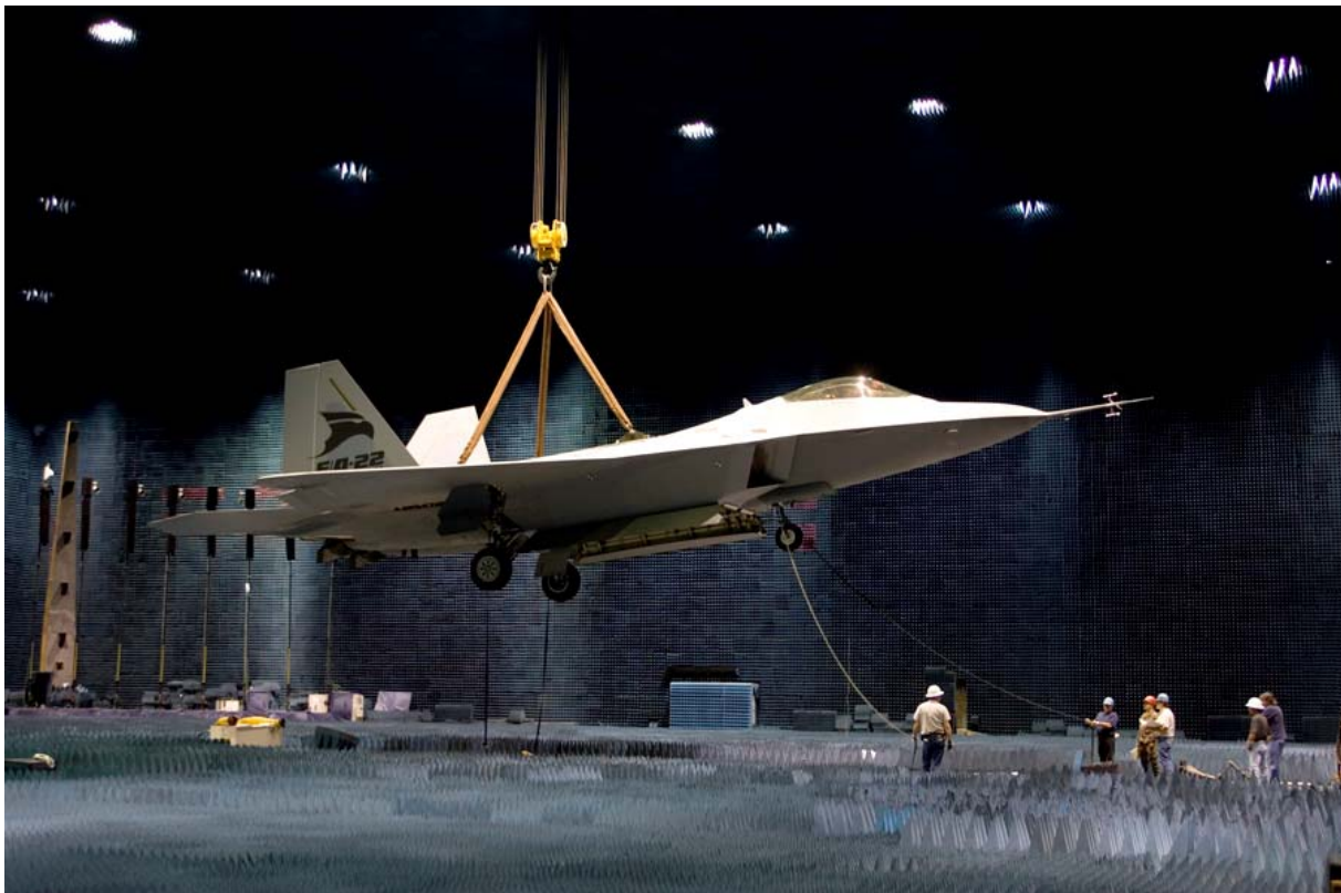
Figure 6-6: ISTF Example 1: Benfield Anechoic Facility – (USAF Photograph).
