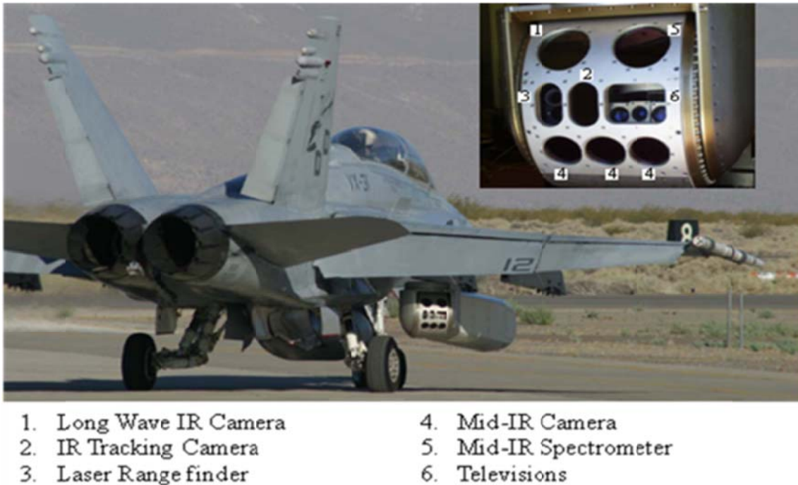
Figure 3-27: Air-to-Air TIGER Pod Mounted on F-18 – (NAVAIR Photo).
