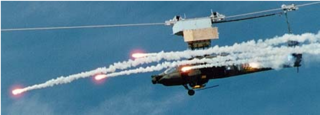
Figure 3-24: Flare Testing Using a Cable Car – (U.S. DoD Photo).
