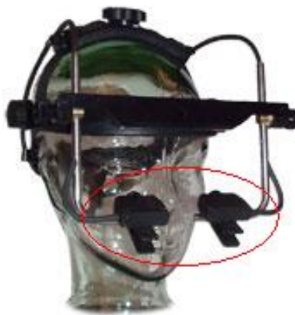
Figure 2: Eyelink II, the red circle highlights the pupil camera and infra red illuminator. With the permission of SR Research Ltd, Ontario, Canada.
