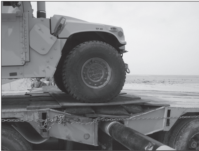
Braces underneath the trailers prevented their suspensions from giving when traffic crossed.
