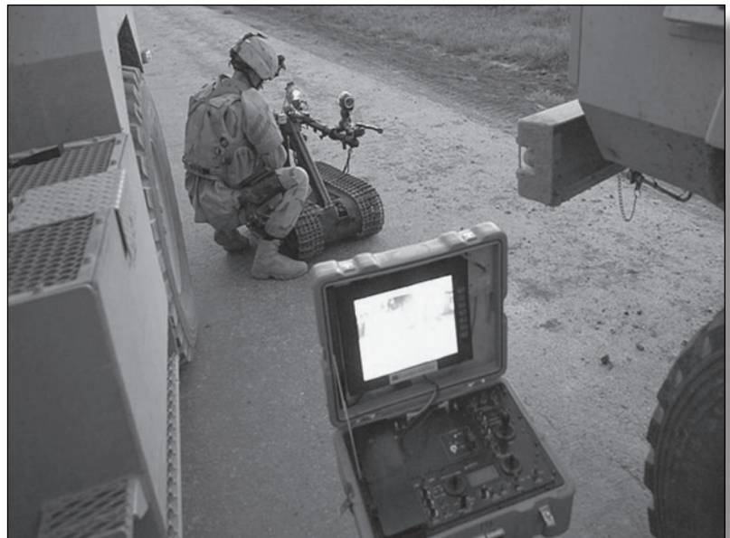
A Soldier prepares an explosive charge to place on a robot to blow an IED in place.
