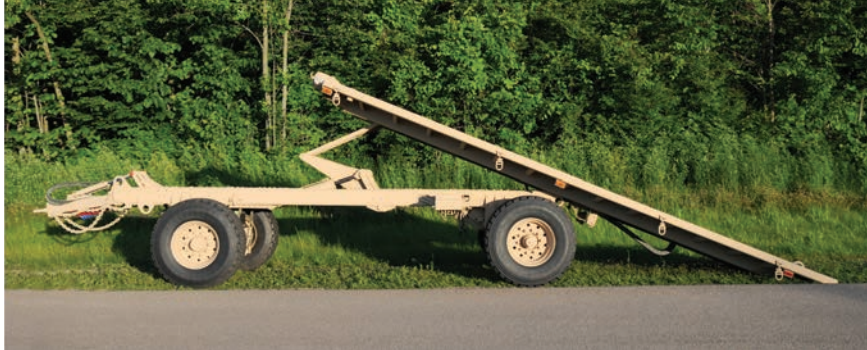
Figure 25: TILT prototypes drive on angle will be reduced by one to two degrees on the production version.
