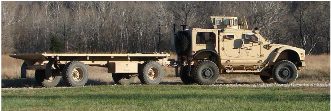
Figure 49: MATV Tow Empty 14T TILT. The unloaded TILT was towed around the demonstration sites behind the AMK36 and an unloaded MATV, at low speed on a one-half mile, mainly flat area without any apparent issues.
