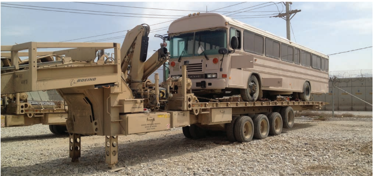
Figure 16: The trailer's long bed is well suited for transportation of long vehicles such as a school bus.
