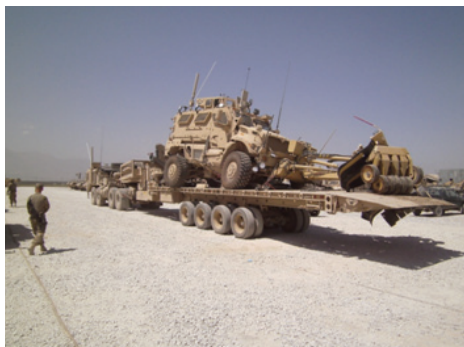
Figure 11: JRaDS 40T with its tailgate down transporting MRAP vehicle with a mine roller attached.
