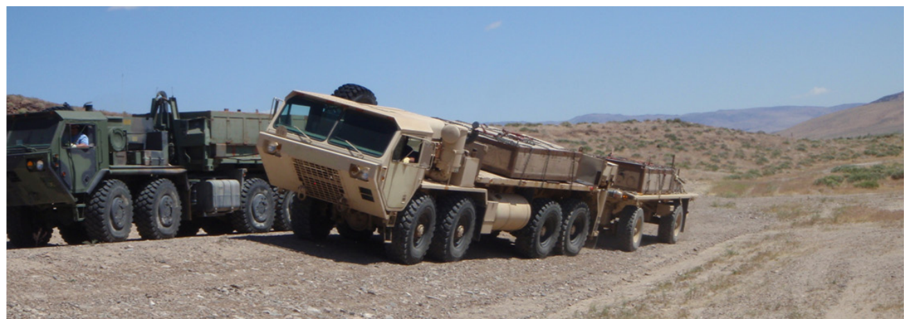
Figure 52: Side slope test configuration using U.S. Army Test Operations Procedure (TOP) 2-2-610 as a guide.
