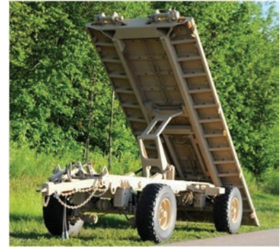
Figure 26: TILT's steep angle design was considered beneficial for quick off-loading capability aiding humanitarian support.
