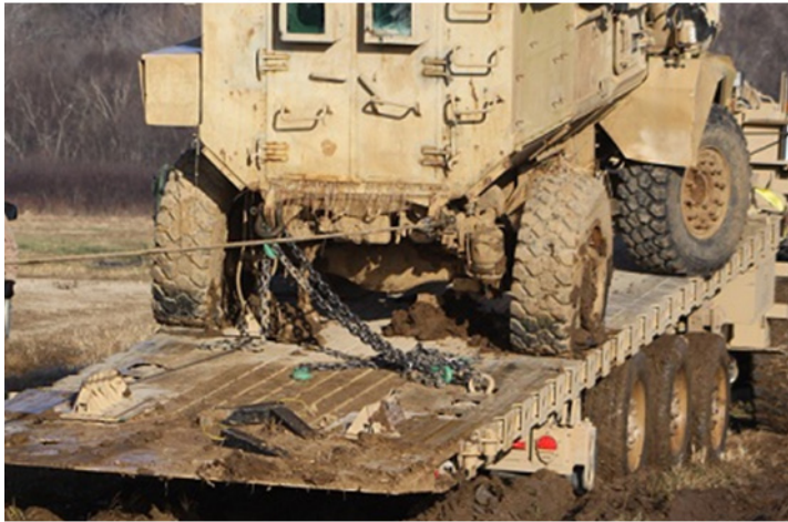
Figure 36: MRAP width compared to trailer deck width.
