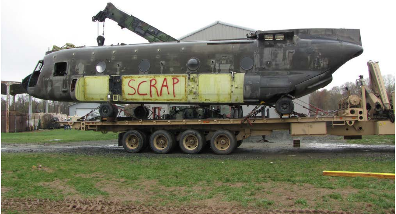
Figure 41: JRaDS trailer proved capable to handle CH-47. CH-47 Boeing Engineering was brought in as experts to assist in developing recovery and loading process of this helicopter.
