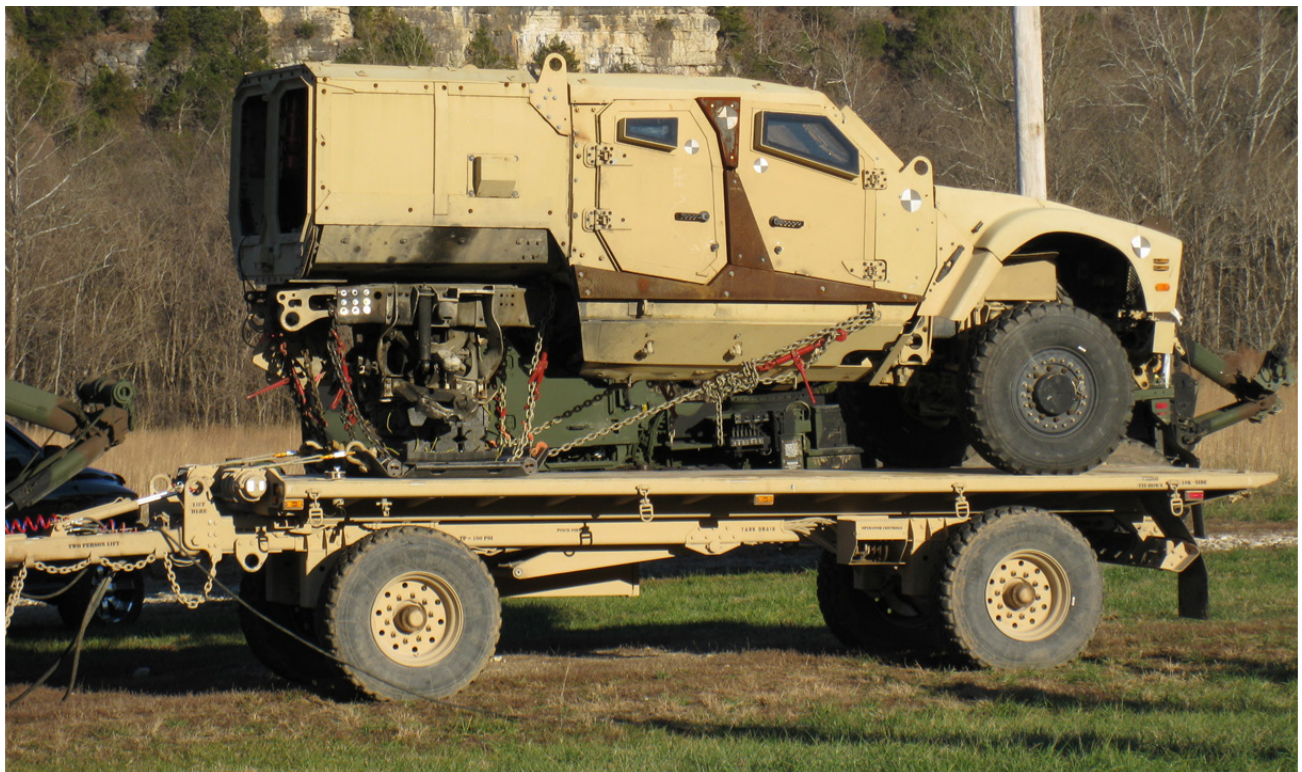
Figure 44: Recover and load MATV missing rear axle assembly.
