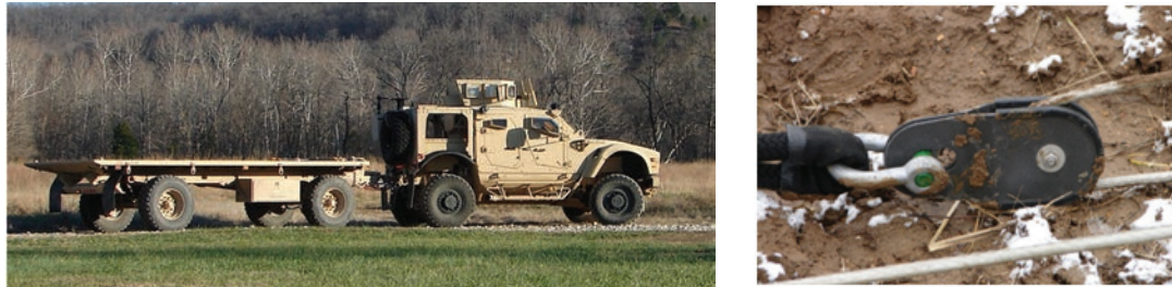
Figure 28: TILT being towed by MATV; TILT's lightweight (six pounds at 60,000 pound capacity) snatch block is off the shelf.
