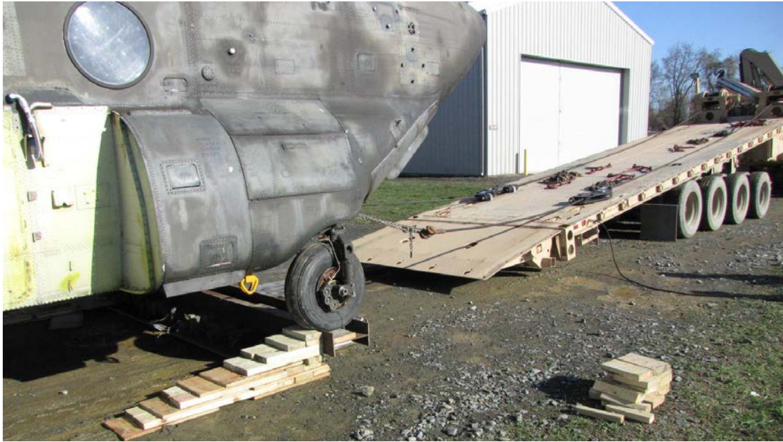
Figure 40: CH-47 loading tech demonstration was requested by theater in response to a recovery need. The JRaDS team prepared loading procedures and sent them to OEF. An I-beam was used to extend trailer width.
