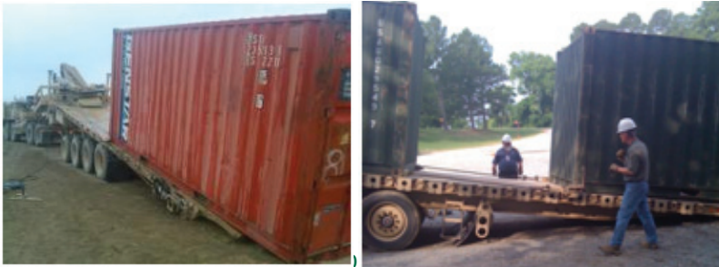
Figure 8: JRaDS trailers (40T left, 34T right) self loading and unloading 20-foot ISO containers using mission equipment.
