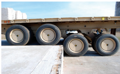
Figure 2: JRaDS 40T – Suspension with demonstrated (18 inch) ability to climb a vertical step.
