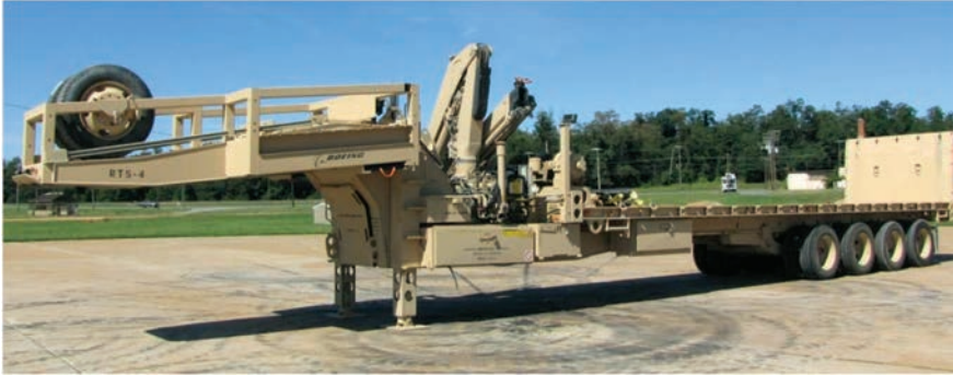
Figure 3: JRaDS 40T showing front "basket" for storage of debris or blown-off vehicle parts.
