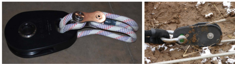
Figure 26: JRaDS lightweight snatch blocks: The one on the left, NSN: 3940-01-602-8022, is for steel cable. The one on the right is for synthetic rope and was only used with TILT trailer.
