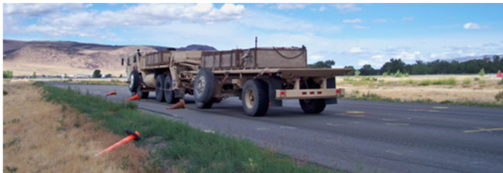
Figure 51: Double-lane-change maneuver test configuration was conducted with the HEMTT M977.
