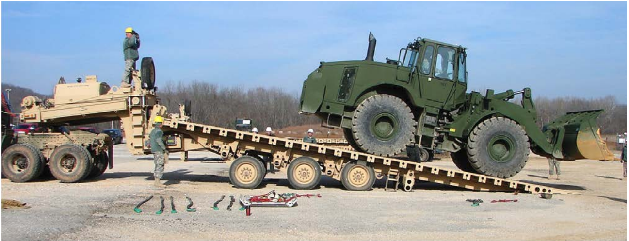
Figure 20: Demonstrated drive-on loading of engineer equipment during operational demo at Fort Leonard Wood – December 2010.
