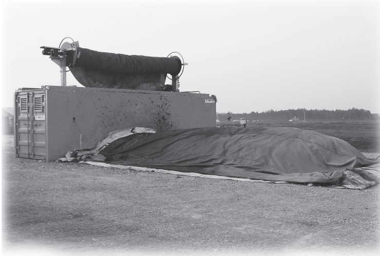
The waste heap is placed on top of the aeration tubes, and the cover is placed over the heap. The temperature and oxygen-monitoring probes are placed through the cover into the heap.
