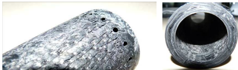
Figure 61: PTAH-SOCAR CMC liner machined for joining with the microfibre shells
