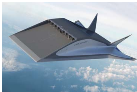
Figure 33 LAPCAT-MR1: outcome of LAPCAT I project for civil Mach 8 transport
