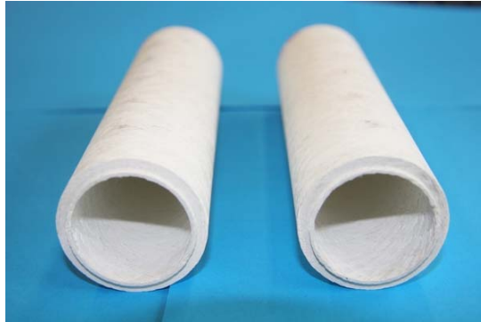
Figure 59: WHIPOX liners manufactured by DLR for transpiration cooling tests at TUM
