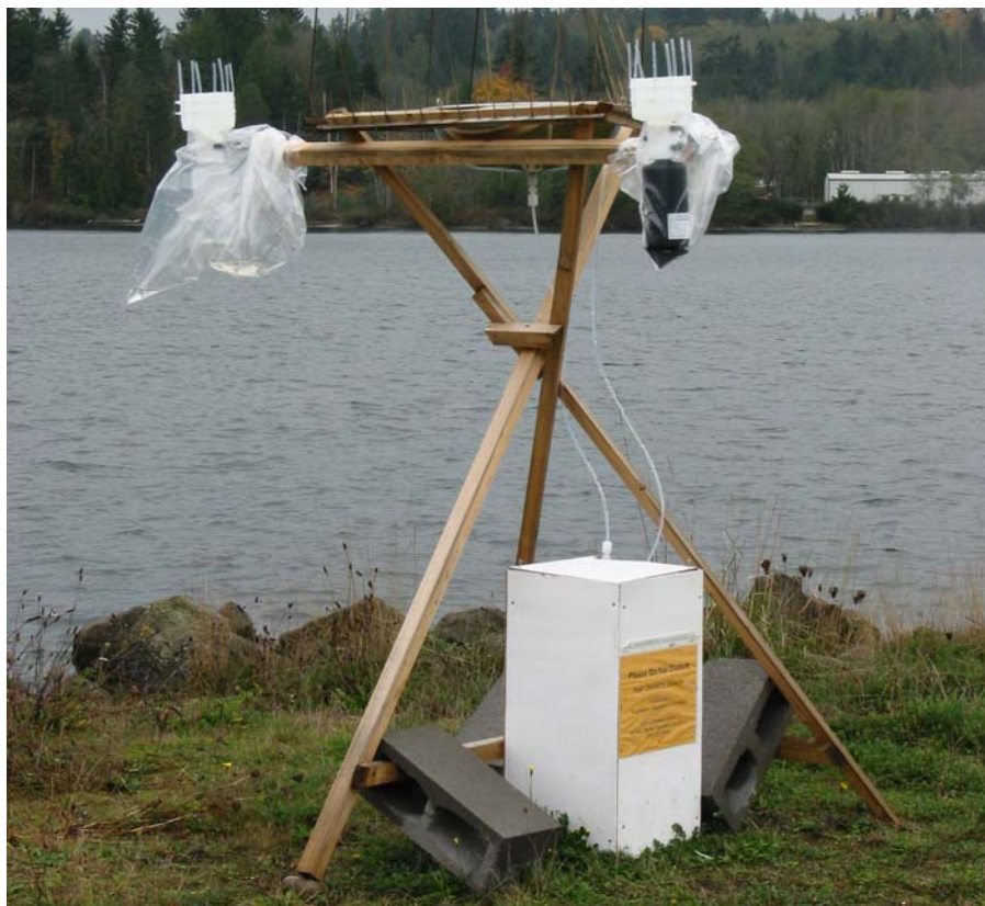
Figure 10. Bulk atmospheric deposition collector with stainless steel funnel in the center draining down into the wood box for organic parameters, clear Teflon® 1L bottles for trace elements (left arm), and opaque Teflon® 1L bottles for mercury speciation (right arm).
