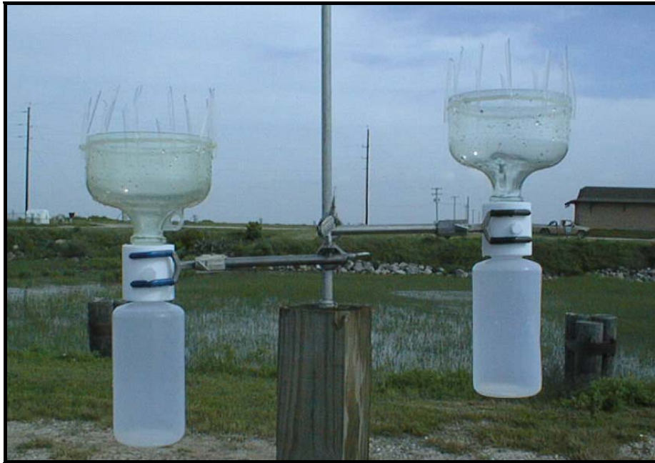
Figure 3. Atmospheric deposition sampler for the collection of trace elements in rainfall and dry deposition.
