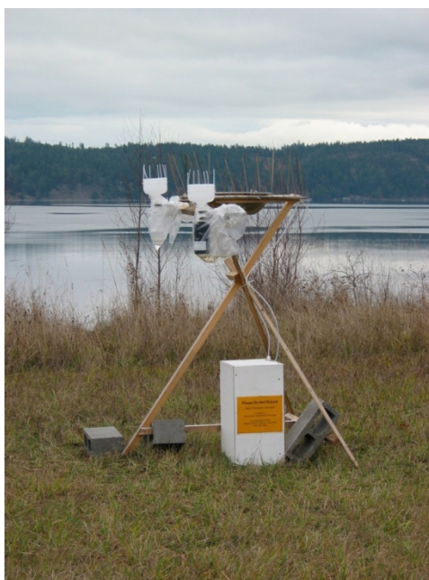
Figure 3. Bulk atmospheric deposition collector with stainless steel funnel in the center draining down into the wood box for organic parameters, clear Teflon® 1L bottles for trace elements (left arm), and opaque Teflon® 1L bottles for mercury speciation (right arm).
