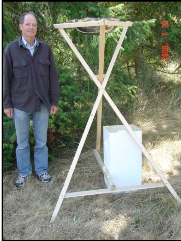
Figure 1. Atmospheric Deposition Sampler for the Collection of Organic Components.
