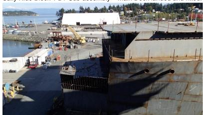
Sally Ride Block 6 Stern – Inspected port and starboard skeg internals prior to yard installing side
